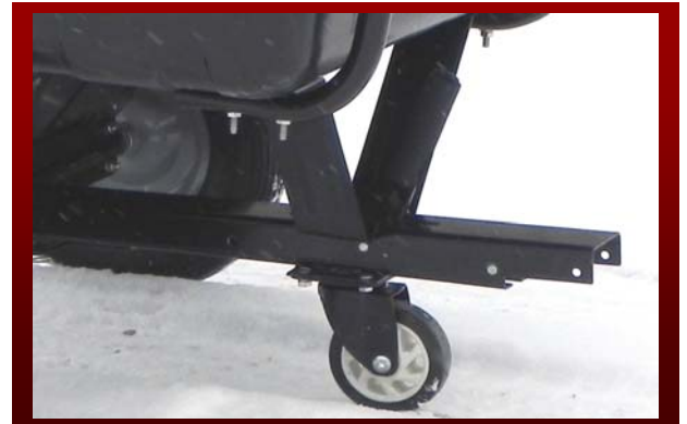
Draw bar folds out of the way and 3rd wheel swivel caster provides stability
