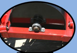
Heavy duty 2" bearings with ductile housing.
