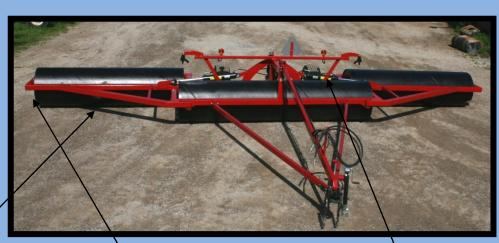
Heavy duty 2" bearings with ductile housing.
