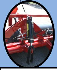
High pressure 4" x 10" cylinder with unique over center lift requires no lock-ups and sequences unfold ie: wings completely unfold before center drum is lowered. Patent Pending
