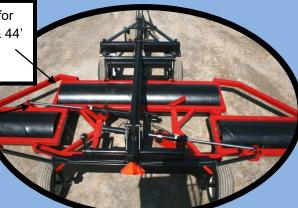
Main drums are 30" x 3/8" wall pipe, 7/16" thick wings drums with 5/16: reinforced end plates and 2" greaseable pins for wing hinge.
