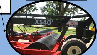
Over - centering four-bar lift assembly requires no lock-up's for transport.
