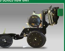
The 25 Series row unit utilizes ductile cast parallel arms for long-term row unit stability. 15", 4mm blades turning on 205 triple-lip sealed bearings ensure long life and accurate seed depth. Blades are offset ½" to slice residue and form a perfect seed trench.
