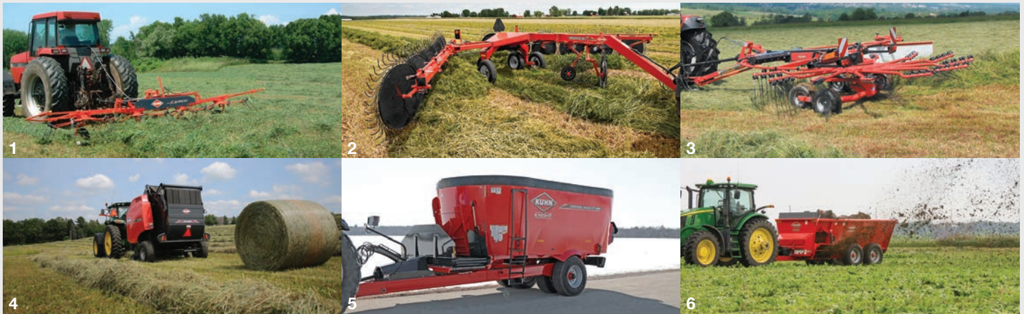
1. Tedders - 2. Wheel Rakes - 3. Rotary Rakes - 4. Mergers - 5. Balers - 6. TMR Mixers - 7. Manure Spreaders - 8. Tedder/Rake Combination
