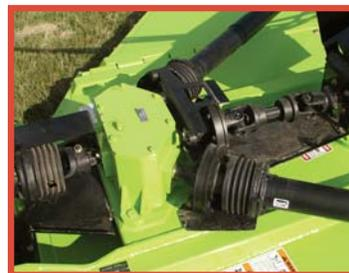
**Forward Mounted Slip Clutches**
