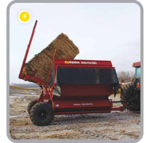
The Twine Sickle™ cuts the twine and the bale is dropped loosely into the tub (the loose consistency helps with uniform processing).
