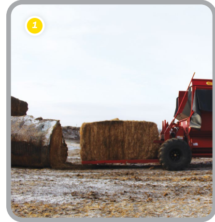
The vertical bale lift is a 2 stage lift system where the first stage of the process lifts the bale straight off of the ground. Little space is required to accommodate this design.
