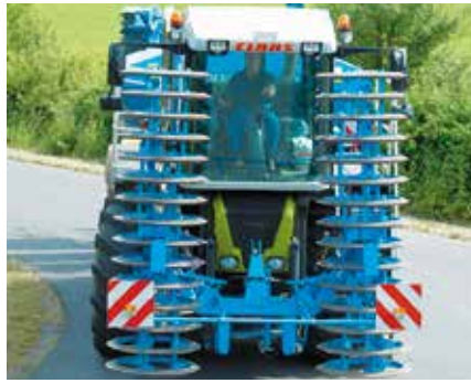
The foldable FEP during transport
