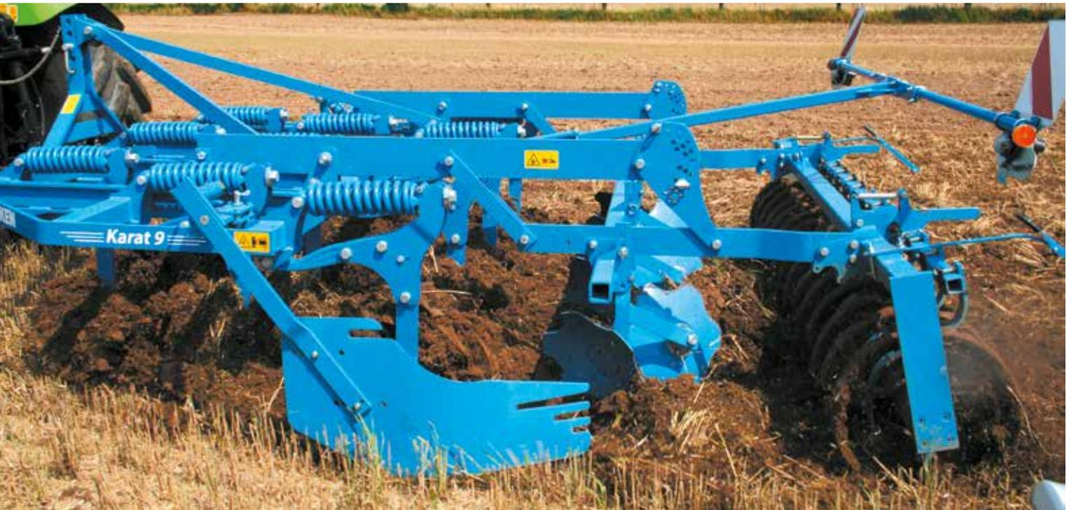
The Karat 9 intensive cultivator is available in working widths of three to seven metres, of which the tines, are arranged on the cultivator frame with an average line distance of about 28 cm to achieve thorough mixing of soil and straw. The symmetrical tine arrangement effectively prevents lateral pull during work.
