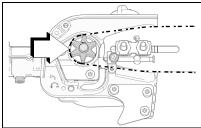
Hold the bar nose up. Install guide bar cover (D). Install the guide bar nuts (A). Tighten the rear nut first, then tighten the front nut. Install and tighten the guide bar cover screw (B)
