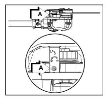
Note: The automatic oiler is preset to deliver a sufficient oil discharge volume during normal operating conditions. During heavy or dry cutting conditions, the oil discharge volume may be increased to assure adequate lubrication. If oil is leaking from the bar cover area, reduce the oil discharge volume. Refill the oil reservoir with each tank of fuel.
