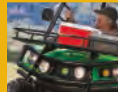
Front hood rack Generously sized rack (48" long, 13.5" wide by 3.5" deep) will carry up to 100 lbs. of gear.
