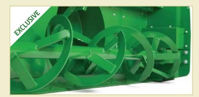
With a 76-inch working width and a sturdy 15-inch auger, you can move heavy volumes of snow with ease. Best of all, the Loader-Mount Snowblower monitors the amount of torque applied to the impeller – an exclusive feature in the industry – allowing the auger to decrease speed when maximum torque is sensed, reducing the chances that the auger overloads the impeller.
