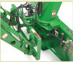
The electronically controlled hydraulic motor adjusts the chute rotation for greater accuracy. Rocker switches are conveniently located in the operator station, so you can adjust chute rotation and angle from the comfort of your tractor seat.
