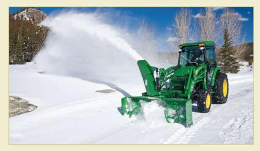
The hydraulic power supply for the SB2176 is provided by a rear hydraulic 3-point mounted power pack, helping to take the strain off of your tractor's hydraulic system. Optional suitcase weights (shown) offer additional ballast to the rear of the tractor.
