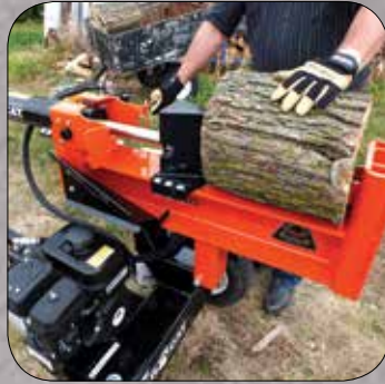
Unique wide-wedge design for quick splitting
