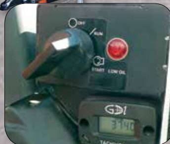
Tach/hour meter is standard on Model CH8720iH
