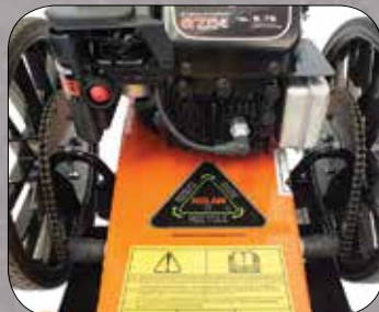
Heavy-duty transmission with chain driven wheels
