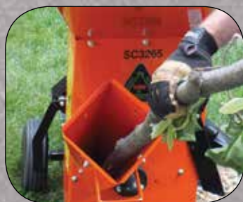
Diamond-shaped chipping chute accommodates irregular-shaped branches
