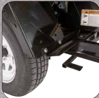
Convenient foot pedal easily engages belt
