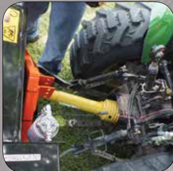
3-point hitch mount hook up
