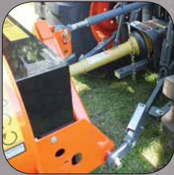
Cat. 1, 3-point connection from 15-60 hp models
