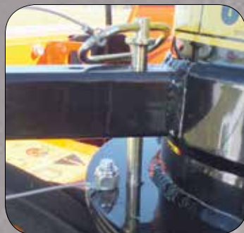
Easy pull discharge chute pin
