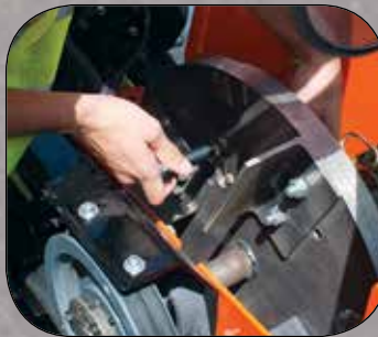
Rotors are easily accessible for quick blade service
