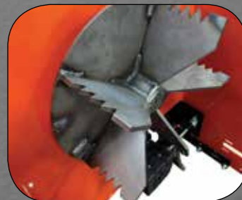
New serrated fan blades for increased material reduction
