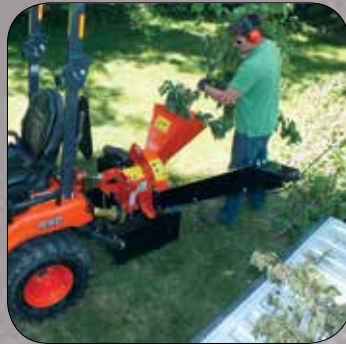
Optional truck loading discharge chute available for CH45540
