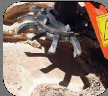
12 hardened carbide tipped cutting teeth
