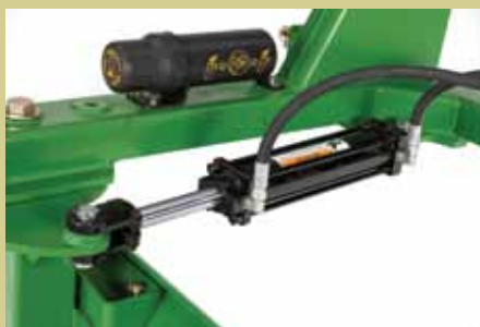
Frontier now offers hydraulic capacity on a medium-duty rear blade with the RB21H Series. You can now adjust blade angle from your operator station, a feature not available before on a rear blade of this duty class.
