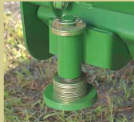
Skid shoes (optional) protect the moldboard cutting edge from hitting low-lying obstructions while cleaning corrals or removing snow.
