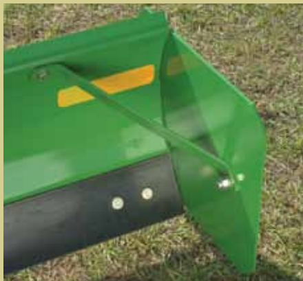
End plates (optional) hold in extra material while dragging it from one place to another, making it an ideal feature for filling.
