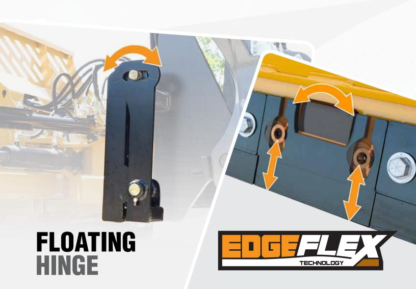
The floating blade hinge is an option on all 3000, 4000, 5000, and 6000 series Angle and Snow Wing Blades. When set up properly, this option gives you 8" of vertical travel at the cutting edge before the loader carrier has to move, allowing you to plow over a speed bump in a parking lot without moving the loader boom, while keeping the blade level with the ground.
