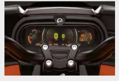
**DIGITAL GAUGE:** Large panoramic 7.8" wide LCD color display with BRP Connect™: allowing the integration of vehicle-optimized smartphone apps such as media, navigation and many others controlled through the handlebars.
