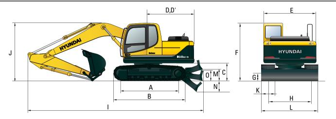
mm (ft·in) 3,170 (10' 5") A Tumbler distance B Overall length of crawler 3,960 (13' 0") **C** Ground clearance of counterweight 1,055 (3' 6") D Tail swing radius 2,530 (8' 4") D' Rear-end length 2,480 (8' 2") E Overall width of upperstructure 2,475 (8' 1") F Overall height of cab 2,980 (9' 9") G Min. ground clearance 460 (1' 6") H Track gauge 1,990 (6' 6") M Ground clearance of blade up 615 (2' 0") N Depth of blade down 675 (2' 3") **O** Height of blade 640 (2' 1")
