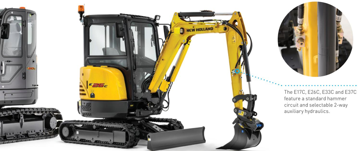
The E17C, E26C, E33C and E37C feature a standard hammer circuit and selectable 2-way auxiliary hydraulics.
