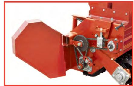
The seeder drive mechanism has been updated to utilize an all roller chain drive train with ball bearing idlers that ensure proper chain tensioning. Number 40 roller chain is used throughout to maintain simplicity.
