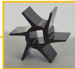
The rear box utilizes a newly designed polyethylene blade type agitator to handle the bulky and chaffy style seeds as well as small seeds at high rates. This new blade agitator is impervious to moisture and is built to provide many acres of reliable seed metering. For specialized requirements, this box can be equipped with an optional brush or cage agitator if needed. Opener spacing is 4".
