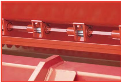
The front Micro-Meter box is designed for the precision metering of legume style seeds such as Alfalfas and Clovers. The exact spacing of the Micro-Meters provides uniform seed distribution for optimum germination.
