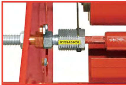
The adjustment of the Micro-Meter has been made user friendly by implementing a new calibration collar and pointer system that requires the use of two wrenches that are provided with the seeder. Seed rates charts are provided to give starting rates for a variety of seeds.
