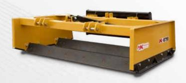
This two in one combination of leveling and scraping makes short work of your grading jobs. The first blade attacks the high spots cutting them down to size, the second blade further scrapes anything the first missed and fills in the hollows. With two blades cutting and filling it takes much less time and fewer passes to achieve the even distribution of material you are looking for.
