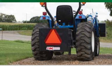
With a material holding volume of 3.5 cubic feet and maximum holding weight capacity of 525 LBS., this new weight box can add up to 575 LBS. of balancing weight to your CAT. 1 3PH. This added weight backs up your tractor by off setting your loader mounted attachments helping to keep your tractor safely balanced during operation.
