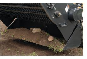
Hydraulic cylinder opens top cover for fast, easy dumping of the large containment bucket.
