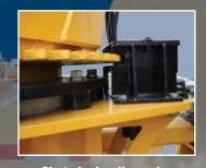
Chute hydraulic engine protected by a damping valve
