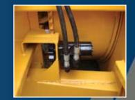
Rotary drum hydraulic engine protected by a damping valve
