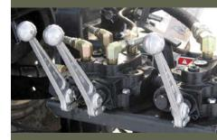
▲ Fingertip hydraulic controls are standard and allows for smooth 4-way tilt, in/out slide and hammer up/down.
