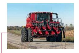
■ Case IH offers folding corn heads in 8-row and 12-row configurations. Capable of folding into transport mode in less than a minute, folding heads dramatically improving transport efficiency, and, ultimately, field productivity.
