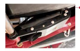
The new air bag suspension system for the center section provides improved flotation and improved range of rotation. Torsion blocks enable the operator to adequately adjust cutterbar pressure for even the most adverse conditions, such as soft fields and wet harvest conditions.
