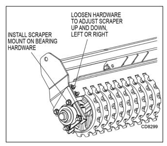
Figure 9. Scraper Installation (Optional)
