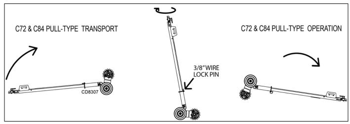
Figure 2. C72 & C84 Pull-Type Transport to Operation
