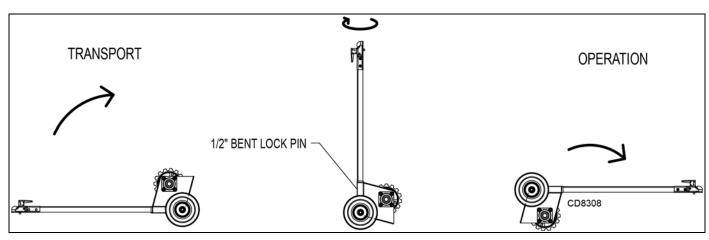
Figure 1. C48T Transport to Operation
