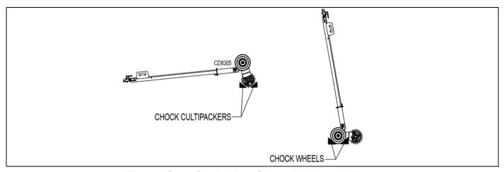
Figure 4. C72 & C84 Pull-Type Storage Positions with Tongue
