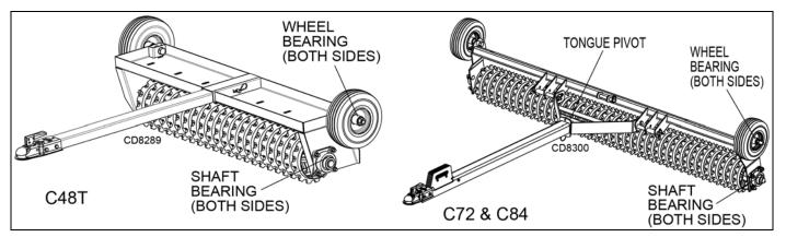
Figure 5. Lubrication Points
