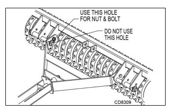
Figure 6. Pull-Type Tongue Installation
