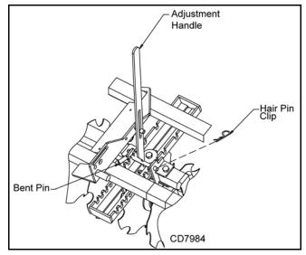
Figure 7. Disc Handle Adjustment (mast plate hidden for picture clarity)
