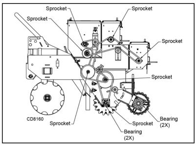
Figure 22. Lubrication Points
