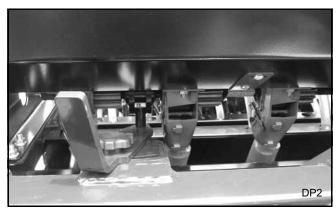
Figure 12. Primary Seed Rate Adjustment Lever
