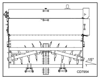
**Figure 2**. Disc in Angled Position (mast plates hidden for picture clarity) (72" Seeder Shown)
