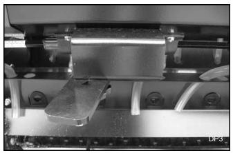
Figure 15. Legume Seed Rate Adjustment Lever
