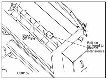
Figure 8. Block Off Plates
