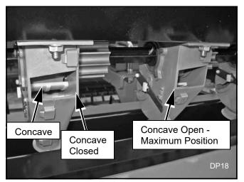
Figure 14. Primary Seed Cup Concave Adjustment
