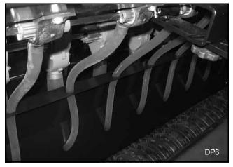
Figure 17. Legume Tubes - Front
