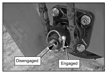
Figure 3. Chain Drive Disconnect
