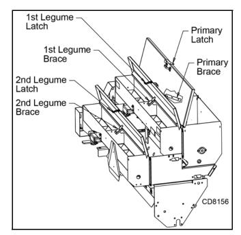
Figure 11. Primary and Legume Braces and Latches
