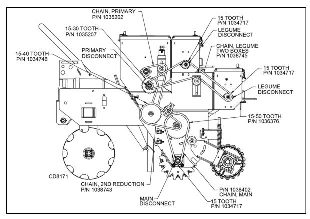
Figure 19. Chain Drive - Two Legume Boxes
