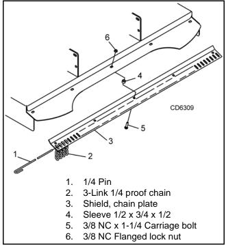
Figure 28. Chain Shield Installed (RDC54 Only)
