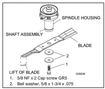
Figure 11. Blade and Spindle Assembly
