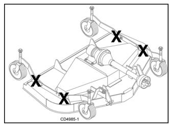
Figure 7. Jackstand Placement
