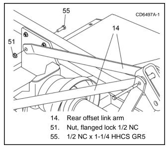
Figure 25. Right Rear Offset Link Installed
