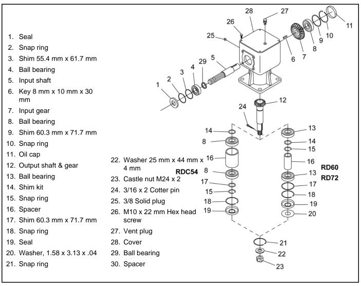
Figure 16. Gearbox Assembly
