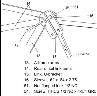
Figure 26. Top Link Assembled
