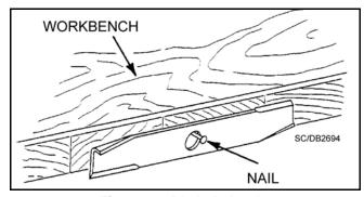
Figure 10. Blade Balancing
