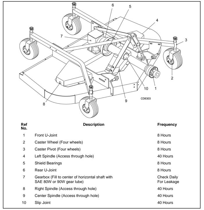
Figure 8Lubrication Points & Chart
