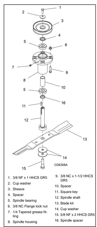
Figure 13. Blade Spindle Assembly
