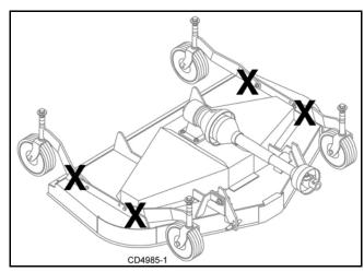
Figure 12. Jackstand Placement
