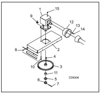
Figure 15. Gearbox Stand Assembly
