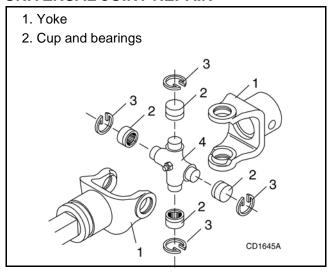
Figure 18. U-Joint Exploded View
