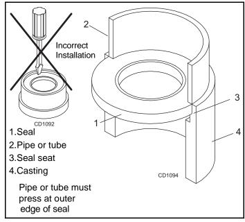
Figure 14. Seal Installation
