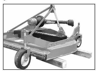
Figure 6. Mower Storage Position
