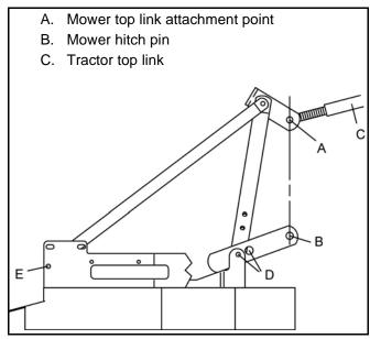
Figure 4. Top Link Adjustment
