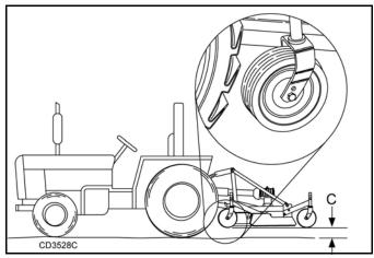
Figure 5. Front Caster Wheel Interference Check
