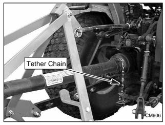
Figure 3Attach Mower to Tractor
