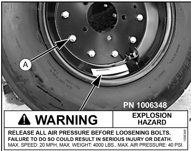
Figure 11. Split Rim Tire Servicing
