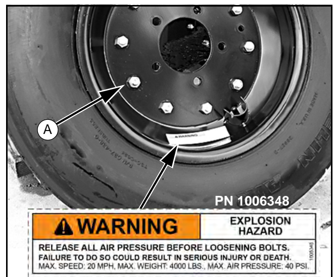
Figure 23. Split Rim Tire Servicing
