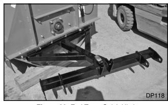
Figure 22. End Tow - Quick Hitch
