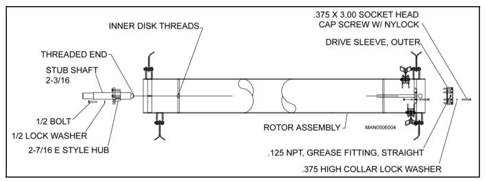
Figure 42. Stub Shaft Assembly
