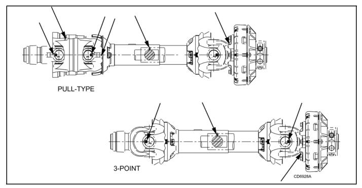
Figure 25. PTO Driveline Lubrication Points
