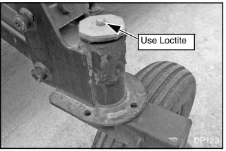
Figure 49. Caster Yoke Installed
