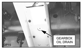
Figure 30. Gearbox Oil Drain Location
