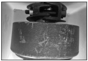
Figure 44. Weasler Automatic Clutch (30K)
