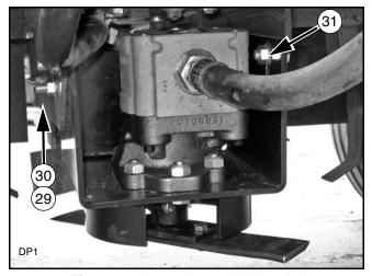
Figure 59. Motor Assembly Installed
