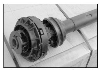
Figure 43. Weasler Modular Friction Clutch (24K)
