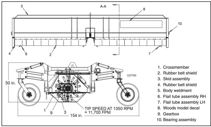
Figure 1. Flail Shredder Principal Components
