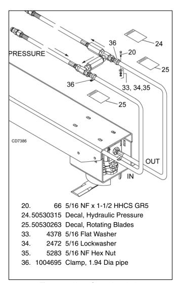
Figure 62. Hose Clamp Installation
