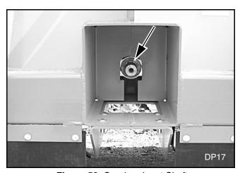
Figure 52. Gearbox Input Shaft
