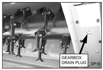
Figure 35. Drain Plug (Underside of Unit)
