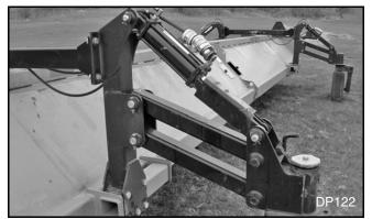
Figure 48. Pivot Tubes, Caster Pivots & Cylinders
