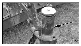
Figure 33. Wheel Caster Bearing Lubrication Points
