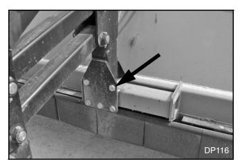
Figure 37. Positioning Wheel Assembly
