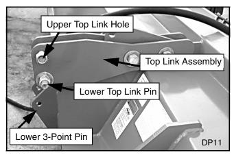
Figure 3. 3-Point Hitch Attachment
