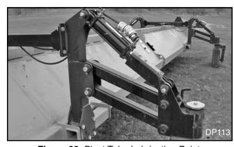
Figure 32. Pivot Tube Lubrication Points
