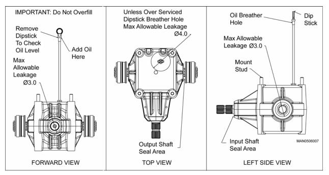
Figure 34. Acceptable Oil Leakage
