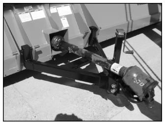
Figure 51. Pull-Type Hitch Installed
