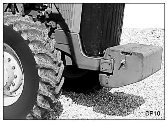
Figure 2. Tractor Front Weight
