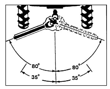
Figure 18. CV Joint Angles
