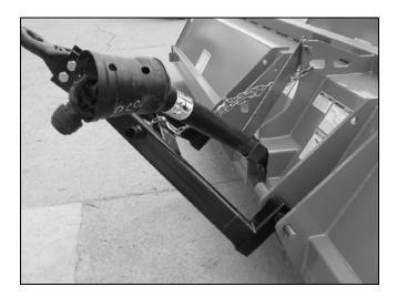
Figure 24. Drawbar and PTO in Transport Position
