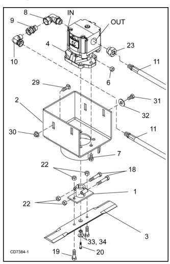
Figure 58. Motor Assembly
