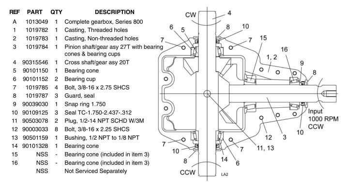
**NOTE:** To separate gearbox halves for servicing, seal guards (8) must be removed first otherwise damage to gearbox housings will occur. Seal guards can be removed by gently prying out of housing with a flat blade screwdriver using the cutout areas machined in the housing to get behind the guards. Use care not to bend guards during removal so they can be reused for reassembly. Replace guards if they are damaged.
