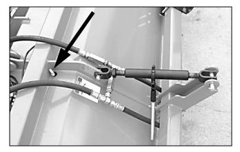
Figure 27. Gearbox Oil Fill Location
