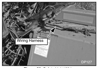
Figure 56. Safety Light Wiring
