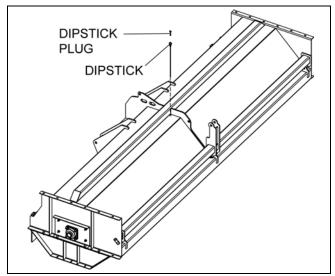
Figure 45. Dipstick Shipping Plug Removal
