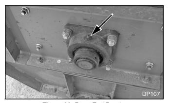
Figure 28. Rotor End Bearing Lubrication Point
