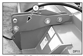
Figure 50. Floating Upper Mast Installed
