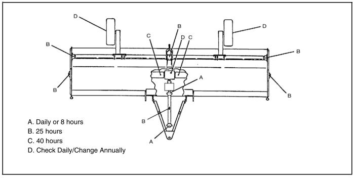
Figure 26. Lubrication Points
