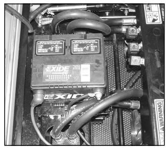
Figure 8. Battery Located Under Seat
