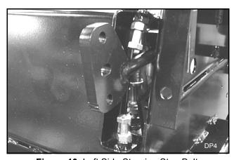
Figure 10. Left Side Steering Stop Bolts
