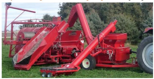
Transfer Style Infeed Auger (Bottom Hopper Style), are designed for loading from dump trucks and trailers, NOT designed for loading directly from semi/ grain trucks.
