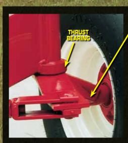
• H&S models 410, 412, 415, 612, 614, and 61 front spindles with structural bracing to withstar from shock loads. The H&S heavy running gears through 622 – utilize thrust bearings to assure smooth turning and straight trailing.
