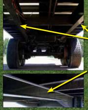
The main frame is made of high quality structural steel 10" I-Beams for the rear and compressed down to 5.13" in the front with full length front gussets.
