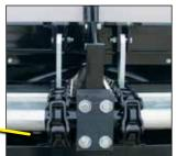
Large 1" steel hydraulic lines to the back of the box drive the **DUAL HYDRAULIC MOTORS** evenly for more power and less shaft stress than a single motor system.
