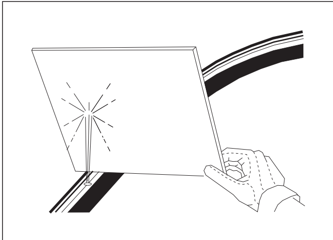
Figure 4-1: Hydraulic Leak Detection
