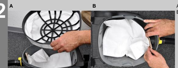
A Remove the main filter basket. Replace the fleece filter bag or paper filter bag (option).
