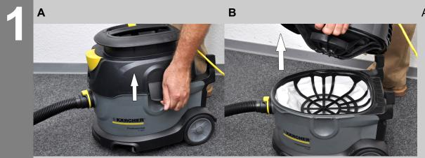
A Release and remove the suction head.
