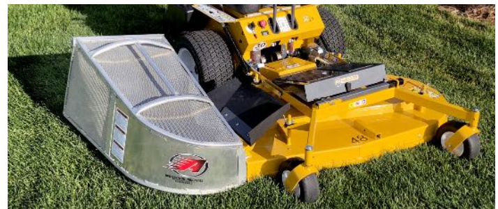
Popular Model R add-on, Accelerator® 3.3 bushel (4.2 cu. ft.) side-mount grass catcher
