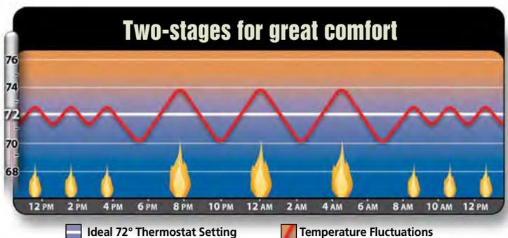
Two-stage gas furnaces offer an immediate level of performance. Operation varies between first and second stage based on demand.
