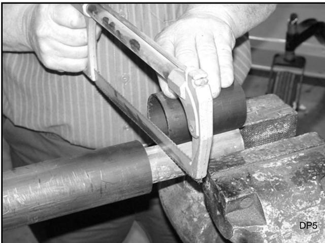
**Figure 7. Cut Shaft to Length**
