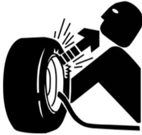
■ Explosive separation of tire and rim parts can cause serious injury or death. Release all air pressure before loosening bolts.
