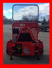
Several protection screens and a "noiseless" chain tightener ensures a safe and good working environment for the user.
