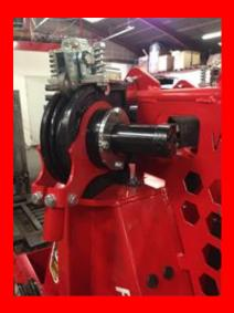
W-8016-EH with optional hydraulic device for unwinding wire rope, relieves the heavy work of pulling the wire out.
