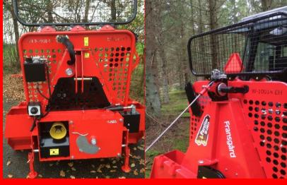
The PTO driven self-contained W-10014-EH with optional hydraulic system assures optimal performance.
