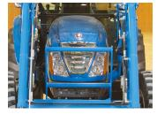
Standard Grille Guard With Loader And Position ROD Protects Grille And Radiator In Loader Applications
