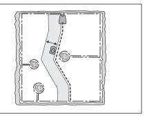
The corridor width is adjusted automatically. Only some times it is necessary to enter manual settings. The corridor width can be set between 0-9. If guide corridor width is set to 0, the product straddles the guide wire. The factory setting is 6 for the boundary wire and 9 for the guide wire.
