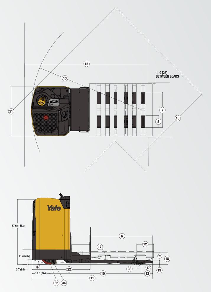
Circled dimensions correspond to the line numbers on the tabulated chart inside the spec sheet. Dimensions are in inches (millimeters).
