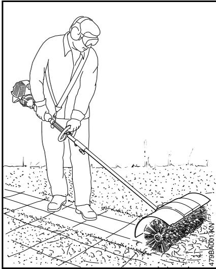
The the KB-KM KombiTool bristle brush is used for cleaning areas and paths, including uneven and jointed surfaces, and natural stone paving.
