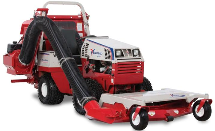
The Ventrac RV602 Vacuum Collection System is for grass and leaf collection, and it consists of three primary components:
