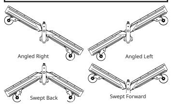
Angle the blade wings to the right or the left to push material to that side. Sweep the blade wings back to push material to both sides for single pass clearing of sidewalks or paths. Sweep both blade wings forward to clear areas without the need for repeated cleanup passes.
