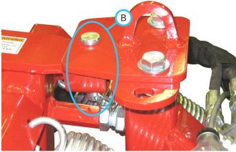
For heavy dozing, the pin can be installed in the lockout hole (B) to lock the blade trip mechanism. This position should only be used for digging or scraping at very slow speeds.
