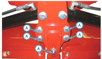
7. Sliding the center frame left or right in relationship to the center hinge shaft will raise or lower the outside corners of the blade wings. Moving the bottom to the right will raise the right side of the blade and lower the left side and moving it to the left will do the opposite. It may be helpful to use a jack or hoist to lift the appropriate side of the blade and then tighten the 1/2 inch bolts.
