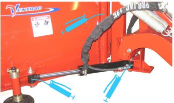
Lubricate the trip/pivot shaft using a spray lubricant.
