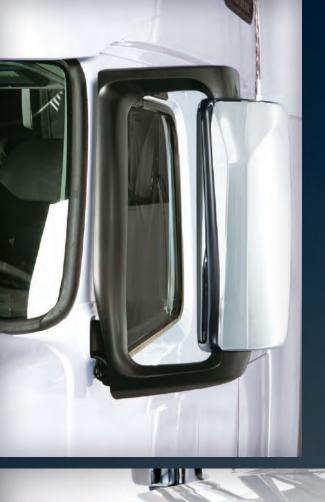
Even in short haul situations, you want to push as little air as possible. So our trucks are wedge-shaped on both horizontal and vertical planes. Smooth sides and minimal surface protrusions help slice though the air to save fuel. Our exclusive Integral Mirror Arm Shroud and A-Pillar Air-Flow Device direct airflow from the windshield and around the mirror arms, reducing turbulence. New sculpted, folding hood mirrors reduce wind resistance as well.
